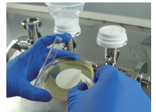
4. Count after the membrane is attached
