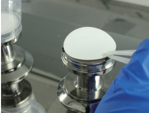
1. Place the filter membrane
