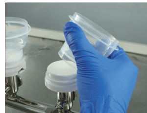
3. Remove the funnel body
