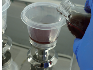
2. Install the filter funnel, add the sample and filter
