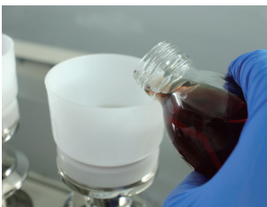
1. Install the incubator, add the sample and filter
