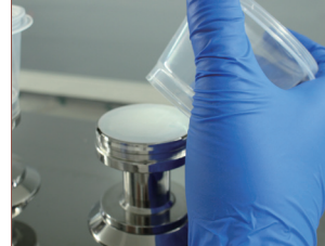
3. Remove the filter funnel
